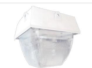
Large size ceiling mount fixture. Vertical lamp HID. Adjustable, 4-way glare guard & "No Bend" conduit entrance. Excellent heat control eliminates heat problems. Housing is die cast aluminum with clear vandalproof polycarbonate refractor. Lamps supplied.
