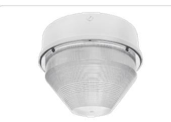
15" round die cast aluminum housing with vandalproof refractor for optimum parking garage light distribution. 150 or 175 w vertical mount Metal Halide or 100,000 hour Induction. Lamp supplied.
