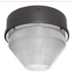
15" round die cast aluminum housing with vandalproof refractor for optimum parking garage light distribution. 150 or 175 w vertical mount Metal Halide or 100,000 hour Induction. Lamp supplied.
