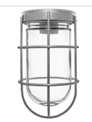
Die cast aluminum construction. Mounts to existing surface or recessed 4" boxes. Adapter plate provided. Medium base socket and a variety of globes. incandescent lamp A21 for 100 Series, PS25 for 200 series. Lamp not supplied.
