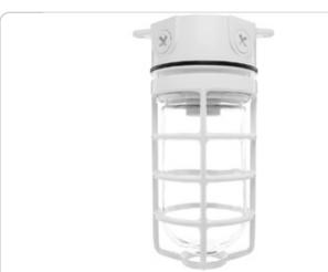
Box mount, die cast aluminum with built-in junction box and sturdy mounting lugs. Medium base socket, 1/2" or 3/4" NPS hub size and a variety of globes. incandescent lamp A21 for 100 Series, PS25 for 200 Series. Lamp not supplied.
