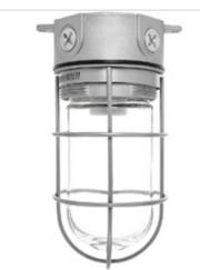
Box mount, die cast aluminum with built-in junction box and sturdy mounting lugs. Medium base socket, 1/2" or 3/4" NPS hub size and a variety of globes. incandescent lamp A21 for 100 Series, PS25 for 200 Series. Lamp not supplied.
