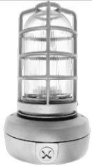
Small cast aluminum housing for 13 and 26 Watt compact fluorescent. Prismatic globe for low glare and even light distribution. Uplight mounted with 1/2" NPS (or 3/4") side and top conduit feed. Specially designed for mounting as an uplight. Lamp supplied.
