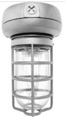
Small cast aluminum housing for 13 and 26 Watt or larger size housing for 32 and 42 compact fluorescent. Prismatic globe for low glare and even light distribution. Fixture mounts to junction box or can be wired inside the housing. Ceiling mounted with 1/2" NPS (or 3/4") side and top conduit feed. Lamp supplied.
