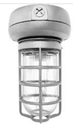
Small cast aluminum housing for 13 and 26 Watt or larger size housing for 32 and 42 compact fluorescent. Prismatic globe for low glare and even light distribution. Fixture mounts to junction box or can be wired inside the housing. Ceiling mounted with 1/2" NPS (or 3/4") side and top conduit feed. Lamp supplied.
