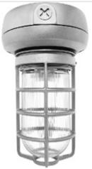
Small cast aluminum housing for 13 and  $2\bar{6}$  Watt or larger size housing for 32 and 42 compact fluorescent. Prismatic globe for low glare and even light distribution. Fixture mounts to junction box or can be wired inside the housing. Ceiling mounted with 1/2" NPS (or 3/4") side and top conduit feed. Lamp supplied.
