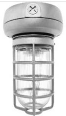
Small cast aluminum housing for 13 and  $2^{\circ}$  Watt or larger size housing for 32 and 42 compact fluorescent. Prismatic globe for low glare and even light distribution. Fixture mounts to junction box or can be wired inside the housing. Ceiling mounted with 1/2" NPS (or 3/4") side and top conduit feed. Lamp supplied.
