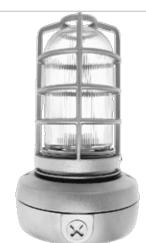
Small cast aluminum housing for 13 and 26 Watt compact fluorescent. Prismatic globe for low glare and even light distribution. Uplight mounted with 1/2" NPS (or 3/4") side and top conduit feed. Specially designed for mounting as an uplight. Lamp supplied.
