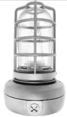
Small cast aluminum housing for 13 and 26 Watt compact fluorescent. Prismatic globe for low glare and even light distribution. Uplight mounted with 1/2" NPS (or 3/4") side and top conduit feed. Specially designed for mounting as an uplight. Lamp supplied.
