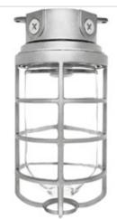
Box mount, die cast aluminum with built-in junction box and sturdy mounting lugs. Medium base socket, 1/2" or 3/4" NPS hub size and a variety of globes. incandescent lamp A21 for 100 Series, PS25 for 200 Series. Lamp not supplied.
