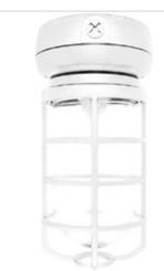
Small cast aluminum housing for 13 and 26 Watt or larger size housing for 32 and 42 compact fluorescent. Prismatic globe for low glare and even light distribution. Fixture mounts to junction box or can be wired inside the housing. Ceiling mounted with 1/2" NPS (or 3/4") side and top conduit feed. Lamp supplied.
