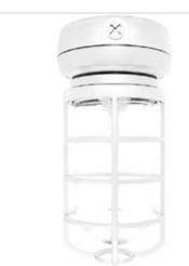
Small cast aluminum housing for 13 and 26 Watt or larger size housing for 32 and 42 compact fluorescent. Prismatic globe for low glare and even light distribution. Fixture mounts to junction box or can be wired inside the housing. Ceiling mounted with 1/2" NPS (or 3/4") side and top conduit feed. Lamp supplied.
