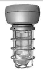
Cast aluminum housing for 50, 70 & 100 Watt HPS and MH. Prismatic globe for low glare and even light distribution. Fixture mounts to junction box or can be wired inside the housing. Ceiling mounted with 1/2" NPS(or 3/4") side and top conduit feed. Lamp supplied.
