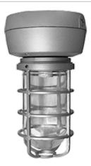
Cast aluminum housing for 50, 70 & 100 Watt HPS and MH. Prismatic globe for low glare and even light distribution. Fixture mounts to junction box or can be wired inside the housing. Ceiling mounted with 1/2" NPS(or 3/4") side and top conduit feed. Lamp supplied.
