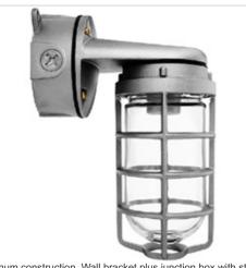
Die cast aluminum construction. Wall bracket plus junction box with sturdy mounting lugs. Medium base socket, 1/2" or 3/4" NPS hub size and a variety of globes. incandescent lamp A21 for 100 series, PS25 for 200 Series. Lamp not supplied.
