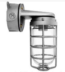
Die cast aluminum construction. Wall bracket plus junction box with sturdy mounting lugs. Medium base socket, 1/2" or 3/4" NPS hub size and a variety of globes. Lamp supplied.
