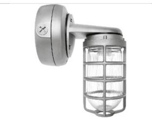
Small cast aluminum housing with study wall mounting bracket for 13 and 26 Watt or larger size housing for 32 and 42 compact fluorescent. Prismatic globe for low glare and even light distribution. Fixture mounts to junction box or can be wired inside the housing. Wall mounted with 1/2" NPS(or 3/4") side and top conduit feed. Lamp supplied.
