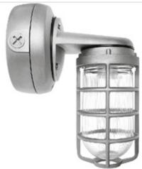
Small cast aluminum housing with study wall mounting bracket for 13 and 26 Watt or larger size housing for 32 and 42 compact fluorescent. Prismatic globe for low glare and even light distribution. Fixture mounts to junction box or can be wired inside the housing. Wall mounted with 1/2" NPS(or 3/4") side and top conduit feed. Lamp supplied.
