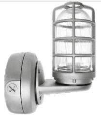
Small cast aluminum housing for 13 and 26 Watt compact fluorescent. Prismatic globe for low glare and even light distribution. Uplight mounted with 1/2" NPS (or 3/4") side and top conduit feed. Specially designed for mounting as an uplight. Lamp supplied.
