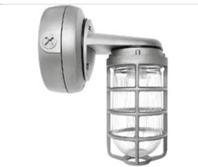
Small cast aluminum housing with study wall mounting bracket for 13 and 26 Watt or larger size housing for 32 and 42 compact fluorescent. Prismatic globe for low glare and even light distribution. Fixture mounts to junction box or can be wired inside the housing. Wall mounted with 1/2" NPS(or 3/4") side and top conduit feed. Lamp supplied.
