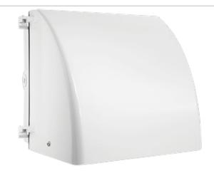
Fully shielded, Full Cutoff compact Wallpack for higher Wattages! 150W HPS & 125W QT P.S. MH. Full Cutoff optics with flat tempered glass lens. Cap/Ignitor cradle and EZ mount knockouts for easy wiring. Lamp supplied.
