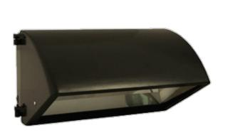
Large cutoff wallpack for 250 Watt HPS or Metal Halide or 120 Watt CFL. All aluminum precision die cast construction with tempered glass refractor. Lamp supplied.
