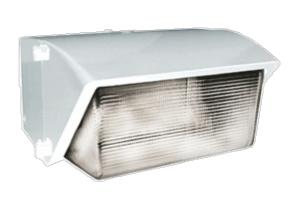
Large wallpack for 400 Watt floods. All aluminum precision die cast construction with tempered glass refractor. Lamp supplied.
