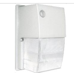
28 thru 42 Watt compact fluorescent Tallpack. Vandal resistant polycarbonate housing. Heavy die-cast aluminum back plate with 1/2" bottom and back conduit opening. Factory installed 120V photocell with bypass cap included. Operating temperature 28w (-20°F), 26, 32 & 42w(0°F). Lamp supplied.
