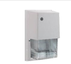
Heavy duty die cast aluminum housing with prismatic glass refractor. HPS and Metal Halide models available with 1/2" bottom and back conduit opening. Factory installed photocell optional. Lamp supplied.
