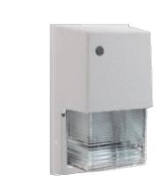
Heavy duty die cast aluminum housing with prismatic glass refractor. HPS and Metal Halide models available with 1/2" bottom and back conduit opening. Factory installed photocell optional. Lamp supplied.
