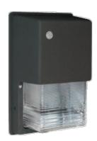
Heavy duty die cast aluminum housing with prismatic glass refractor. HPS and Metal Halide models available with 1/2" bottom and back conduit opening. Factory installed photocell optional. Lamp supplied.
