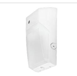
High performance LED tallpack. Covers footprint of most HID Tallpacks. Vandal resistant lens. Precision die-cast aluminum. 0-10V dimmable driver with 120-277V photocell.
