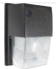
HPS "Tall" Wallpack. Vandal resistant polycarbonate housing. Heavy die-cast aluminum back plate with 1/2" bottom and back conduit knockout. Factory installed 120V photocell with bypass cap included. Glare shield included. Lamp supplied.
