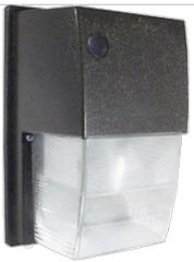
HPS "Tall" Wallpack. Vandal resistant polycarbonate housing. Heavy die-cast aluminum back plate with 1/2" bottom and back conduit knockout. Factory installed 120V photocell with bypass cap included. Glare shield included. Lamp supplied.
