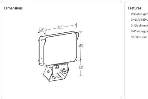
Versatile, general-purpose floodlight 7H x 7V NEMA distribution 0-10V dimming IP65 rating protects against dust and water 50,000-Hour LED lifespan
